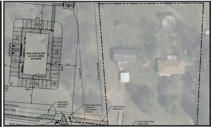
Figure B-3. Site plan excerpt showing the proposed store footprint, fuel canopy/pump area, parking layout, and internal circulation. Source: Concept Site Plan #2.
