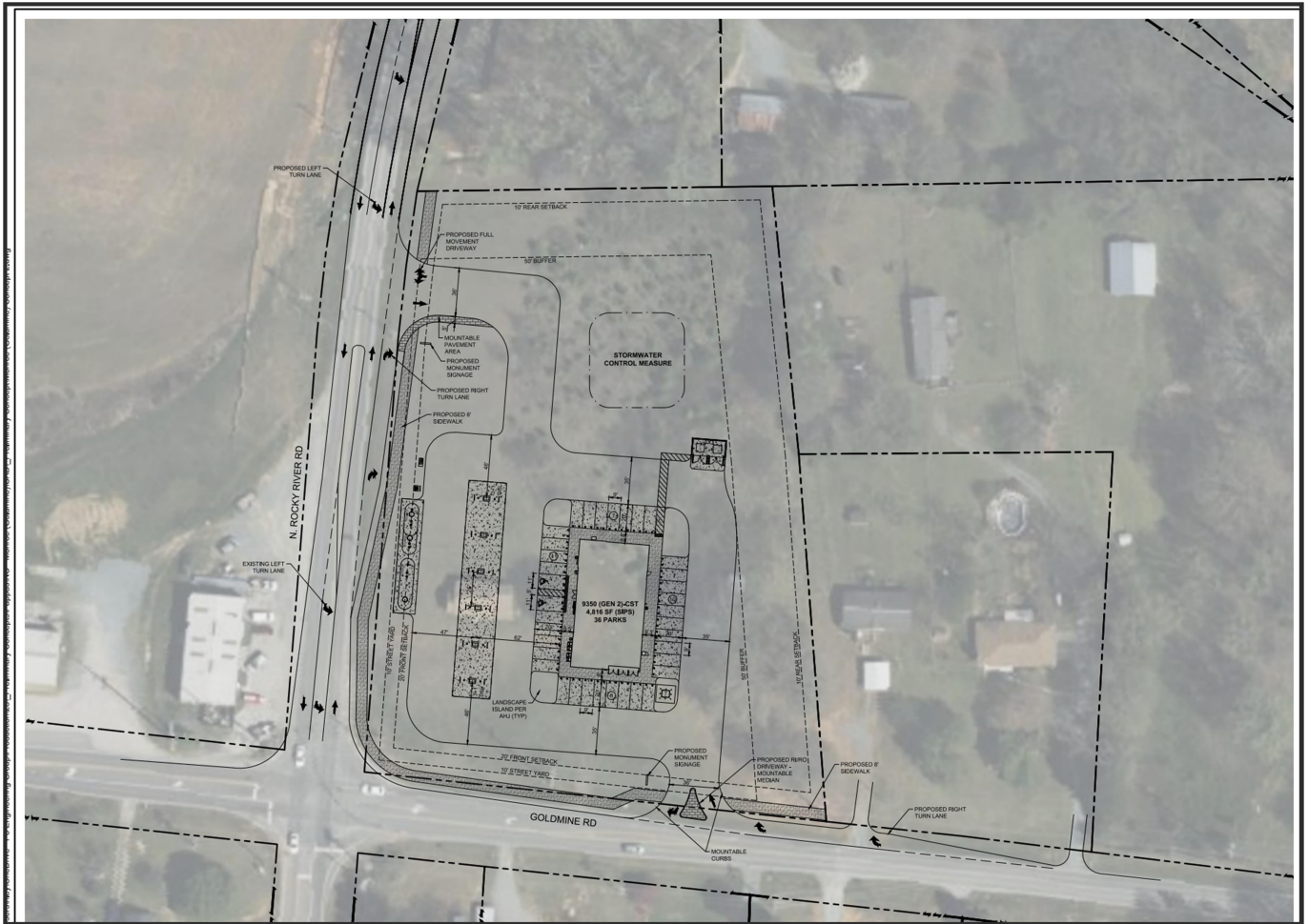
Figure B-1. Conceptual site plan showing proposed convenience store with fuel, parking, fuel canopy, access points, internal circulation, turn-lane improvements, stormwater control measure, sidewalks, and perimeter buffer/setback areas. Source: Concept Site Plan #2, dated 03/05/2026.
