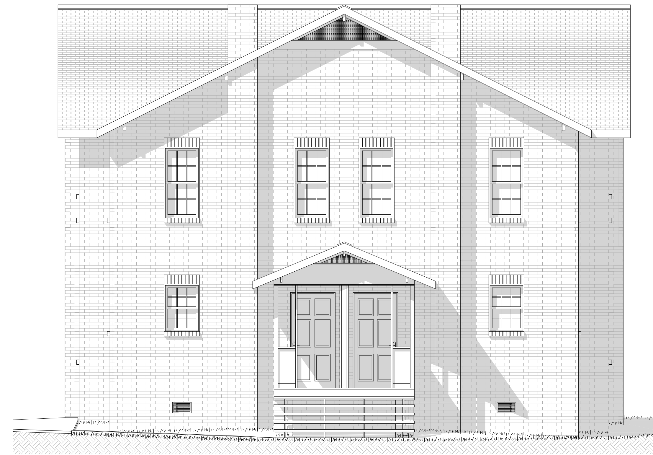
3 REAR ELEVATION - EXISTING CONDITIONS SCALE: 1/4" = 1'-0"
