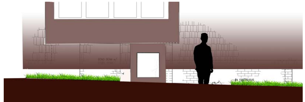
West Wall– New door, areaway and stair
