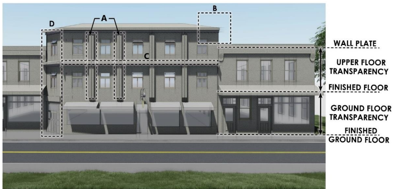
Figure 8.7.1.1. Required Facade Design Elements Example
