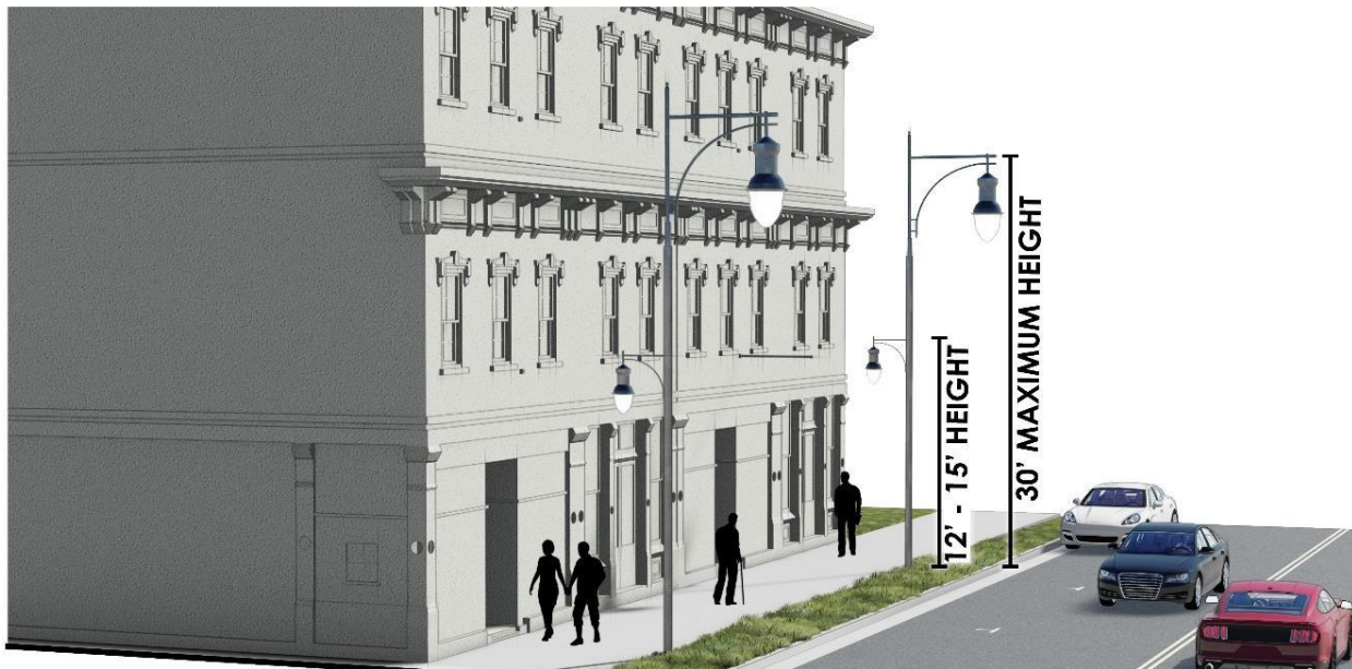
Figure 8.9.1. Light Fixture Height
