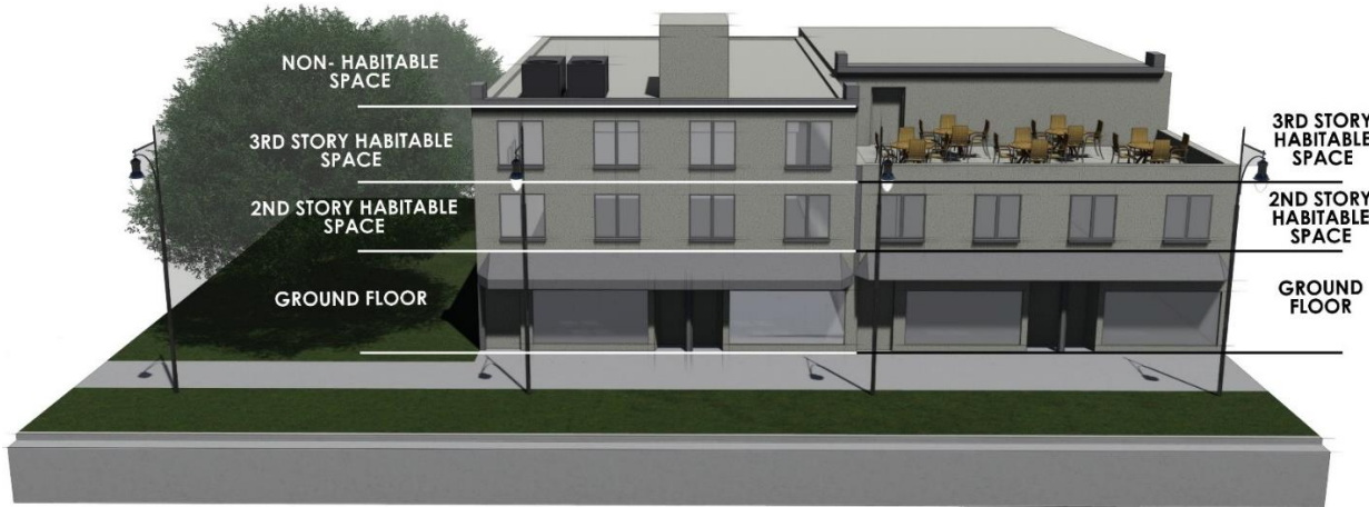
Figure 8.10.3. Building Height Illustrations
